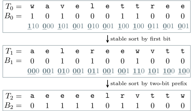
Figure 6: The stable sorting algorithm for T = \text{wavelettreetree} . Below the symbols, we show the corresponding bit in the level’s bit vector and the symbols’ binary representations. The bit prefix used as the sort key is highlighted in bold.
