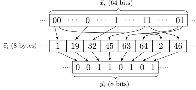
Figure 1: Example of the bit shuffle instruction with selection vector  $\vec{c}$  for the  $i$ -th 64-bit block of the input vector  $\vec{x}$ , producing the  $i$ -th 8-bit block of the result vector  $\vec{y}$ .
